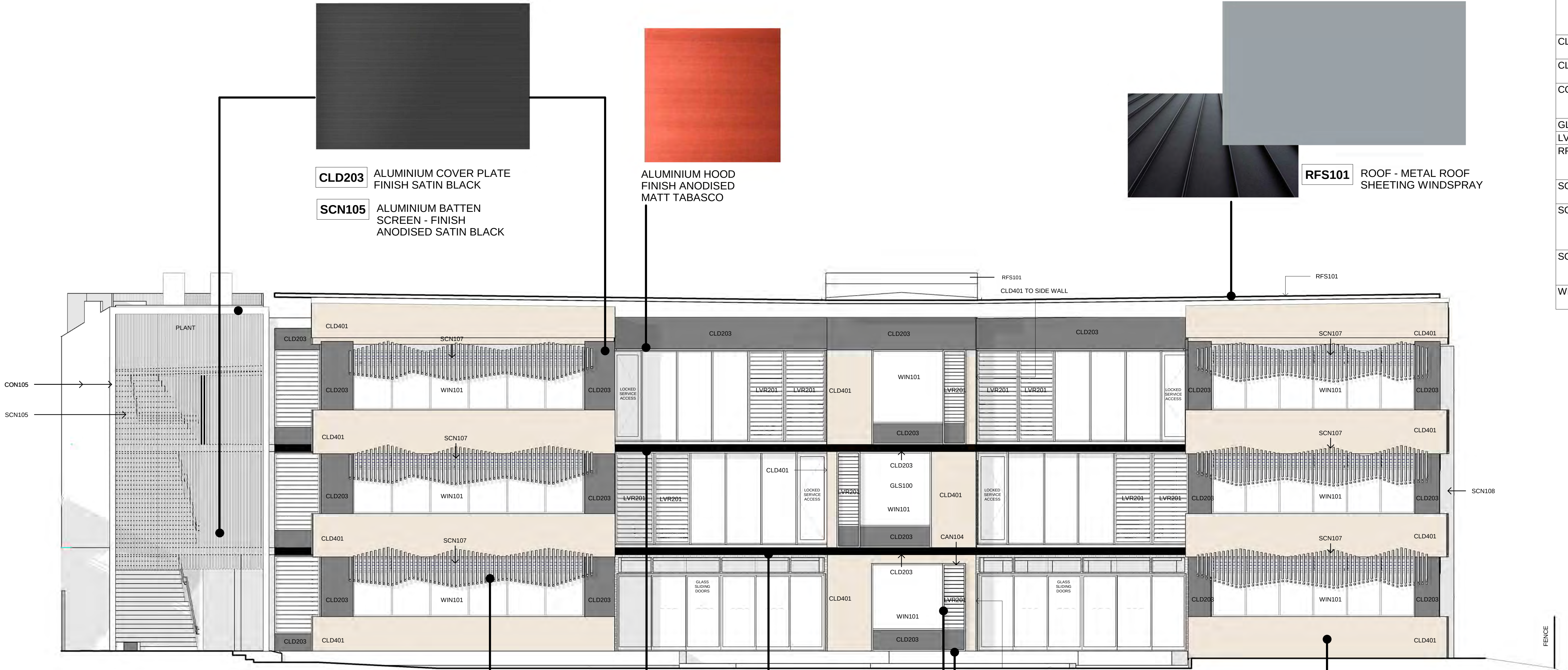
1 BUILDING N - NORTH ELEVATION - MATERIAL FINISHES 1 : 75
